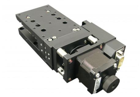
The stage delivers good parallelism (<20  $\mu$ m to the mounting surface), and high resolutions to 1.25  $\mu$ m (full step), 0.625  $\mu$ m (1/2 step), and 0.125  $\mu$ m (1/10 micro step), and repeatability to +/- 0.5  $\mu$ m. Travel speeds are up to 2.5 mm/sec.
