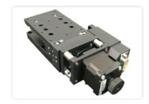
The AZ60-A Motorized Vertical Elevator Stage from Optimal Engineering Systems is a low profile, compact 183.7 mm x 80 mm x 38 mm ~ 42mm (raised), (7.232in x 3.150 in. x 1.496 ~ 1.654 in.) low cost, high resolution, wedge type, vertical elevator stage for applications requiring precise vertical positioning.
